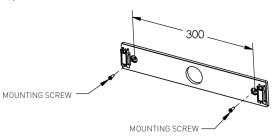
b) Slide the base over the wall bracket.
