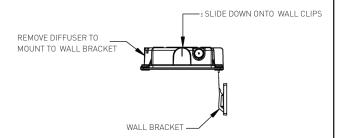
c) Secure the base to the wall bracket.
